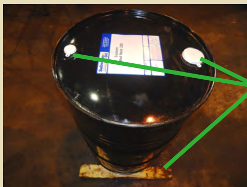
2x4 board placed under bottom chime, parallel to drum’s bungs
